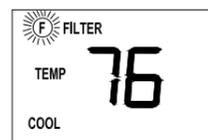
After changing or cleaning the system filter, press and hold the Filter key for 3 seconds. The display will blink, and the counter will be reset to zero.
