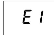
To correct this problem, replace the batteries with 2 new AA alkaline batteries, even if you have recently replaced them. Next, Move the battery out hold any key then place the battery again. You will need to reprogram your thermostat and confirm normal operation.
